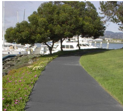
Bike path at shoreline park in Marina Village – 8 feet wide, asphalt
