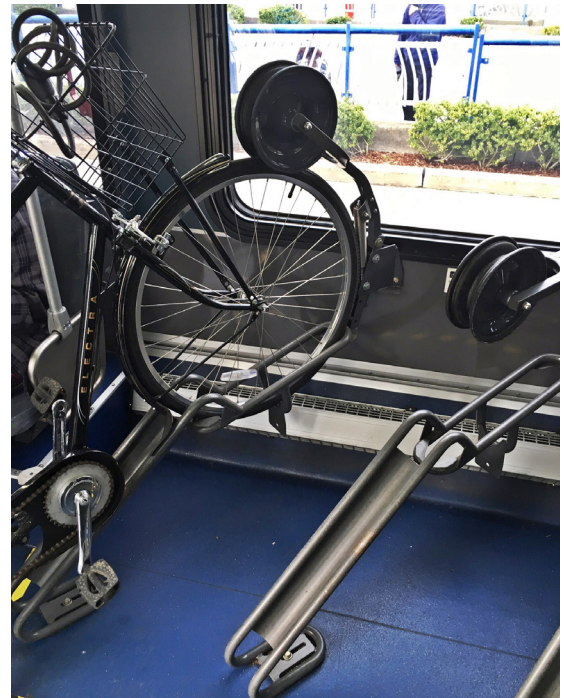
Bus interiors have been modified to accommodate bicycles on Swift Express bus service operated by Community Transit in Washington State. (Photo source: CDM Smith)
