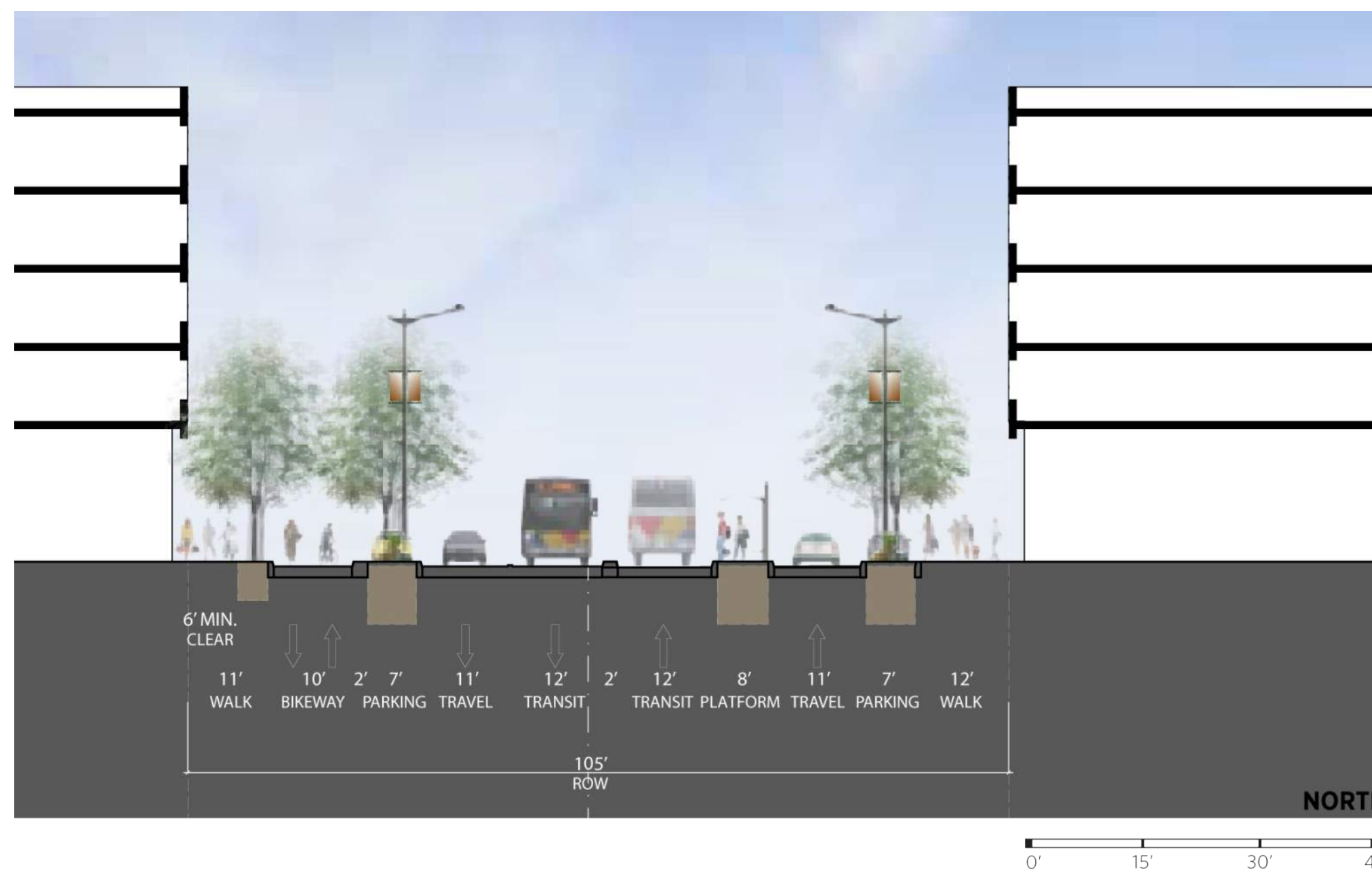
B. RALPH APPEZZATO MEMORIAL PARKWAY - EAST 105' R.O.W. SECTION SECTION REVISED FROM PRECISE PLAN DOCUMENTS
