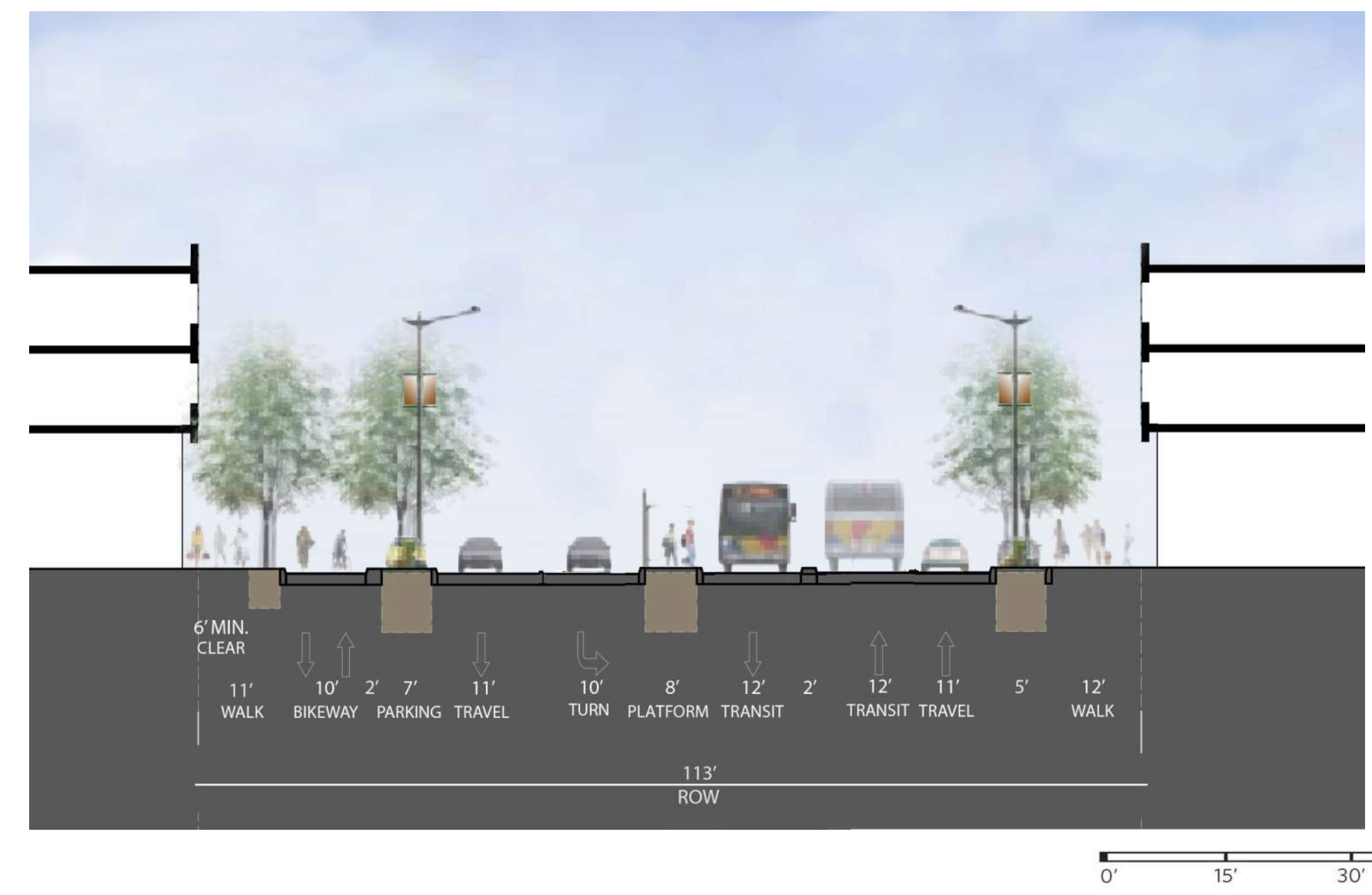
A. RALPH APPEZZATO MEMORIAL PARKWAY EAST 113' R.O.W. SECTION AT MAIN STREET SECTION REVISED FROM PRECISE PLAN DOCUMENTS
