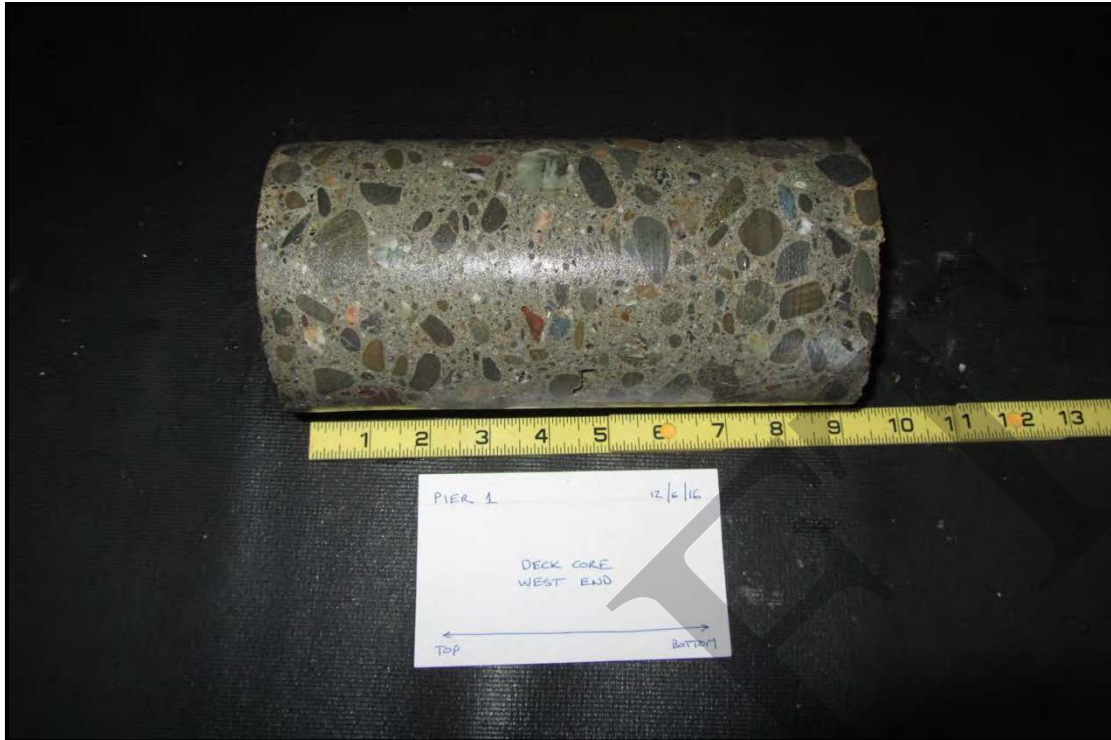
Photo 15: Concrete core sample taken from Pier 1 deck.
