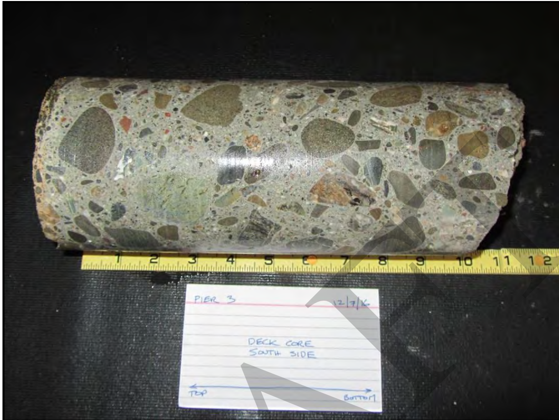
Photo 27: Core sample from deck of Pier 3.
