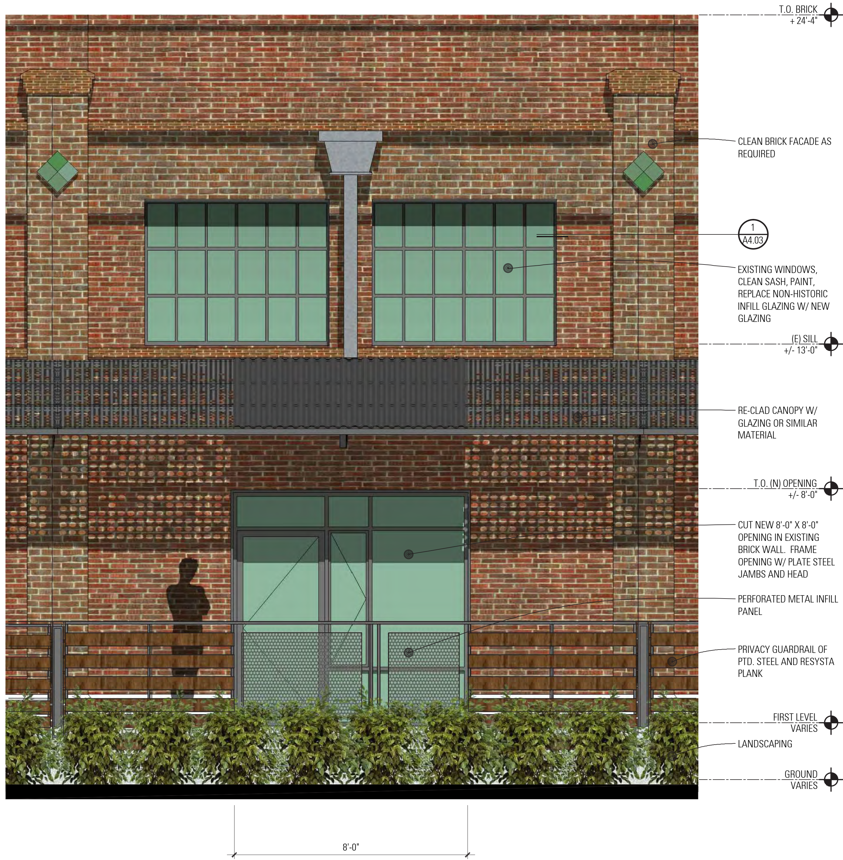
2 A3.06 NEW OPENING IN BRICK FACADE 1/2"=1'-0"
