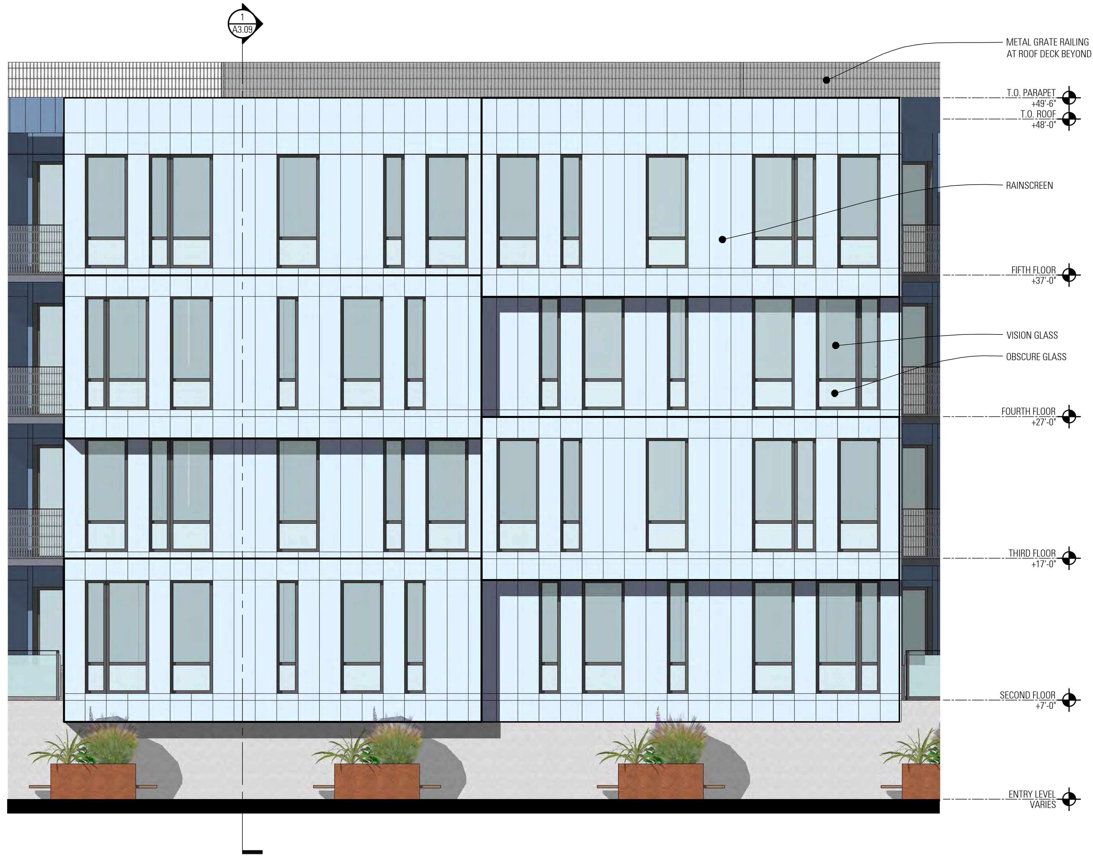
2 A3.09 ENLARGED ELEVATION PASEO BAY 2 1/4"=1'-0"
