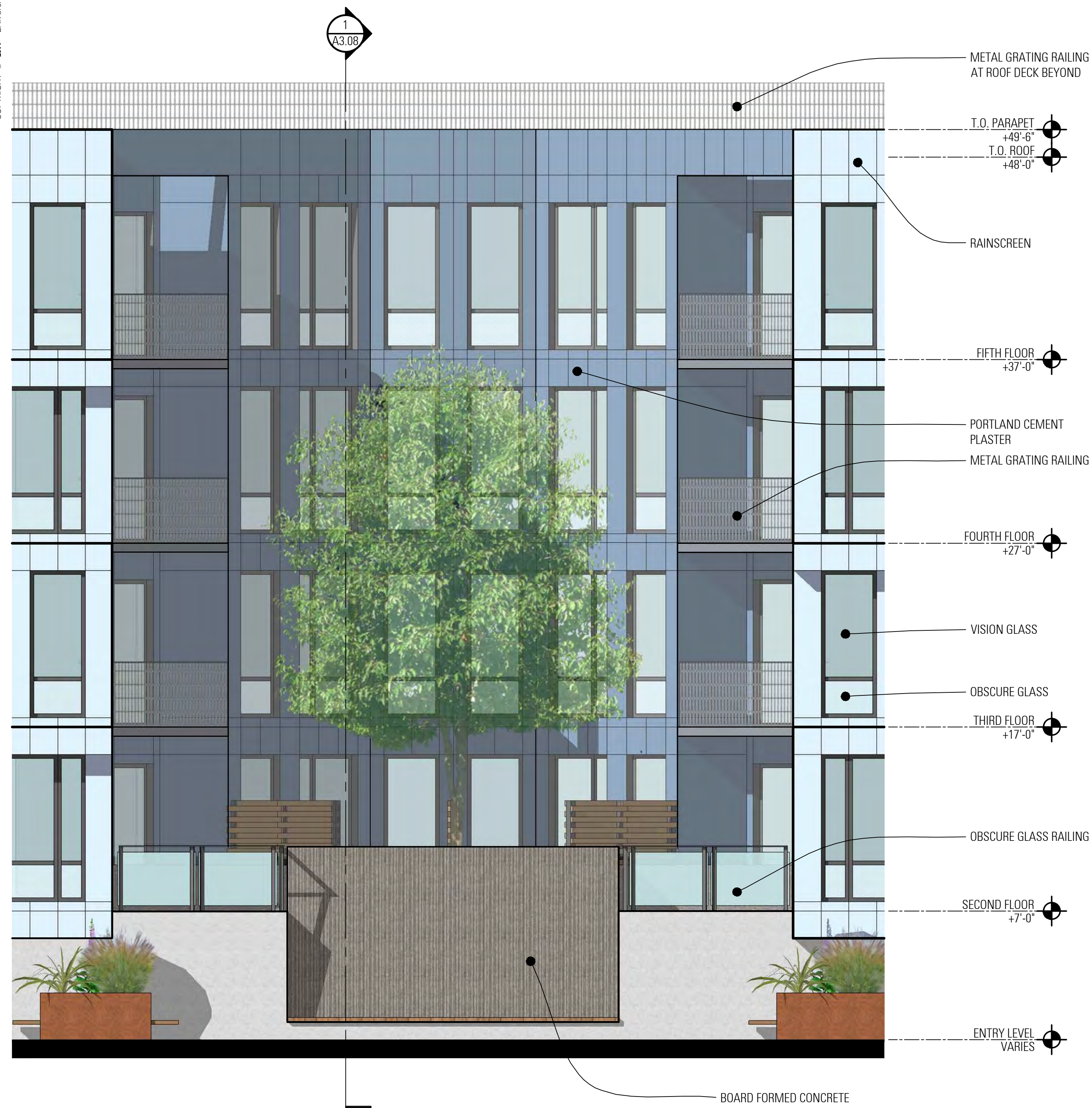
2 A3.08 ENLARGED ELEVATION PODIUM COURTYARD 1/4"=1'-0"
