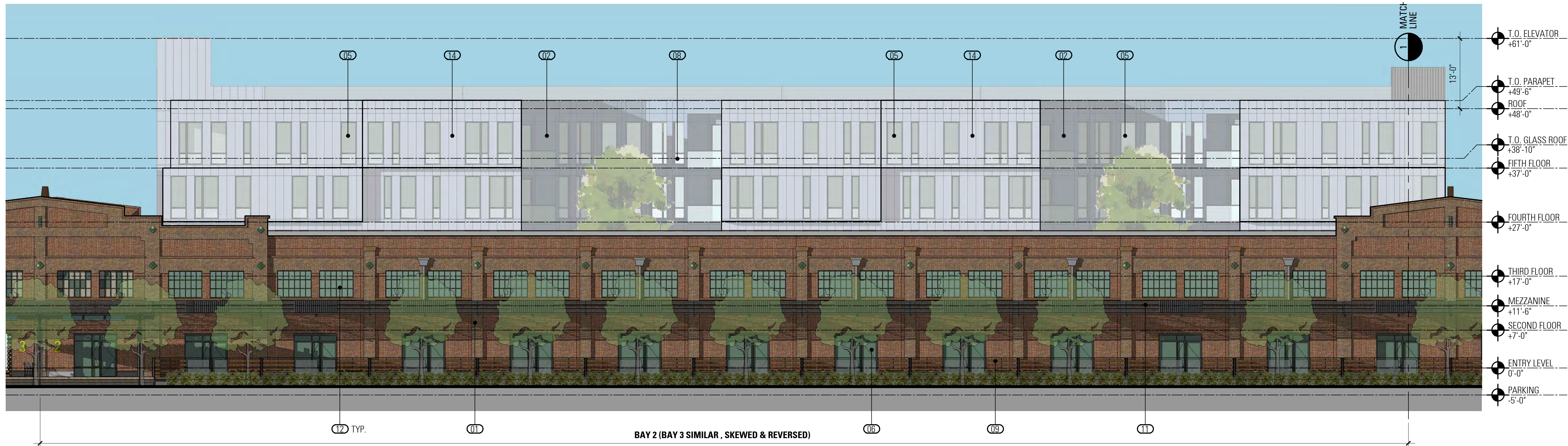
2 A3.03 BAY 2 - ENLARGED NORTH ELEVATION BAY 3 - SIMILAR, SKEWED AND REVERSE 1" = 10'
