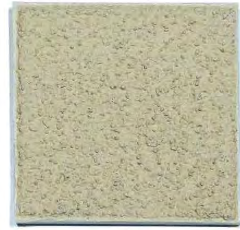
Sand Finish Stucco Field texture
