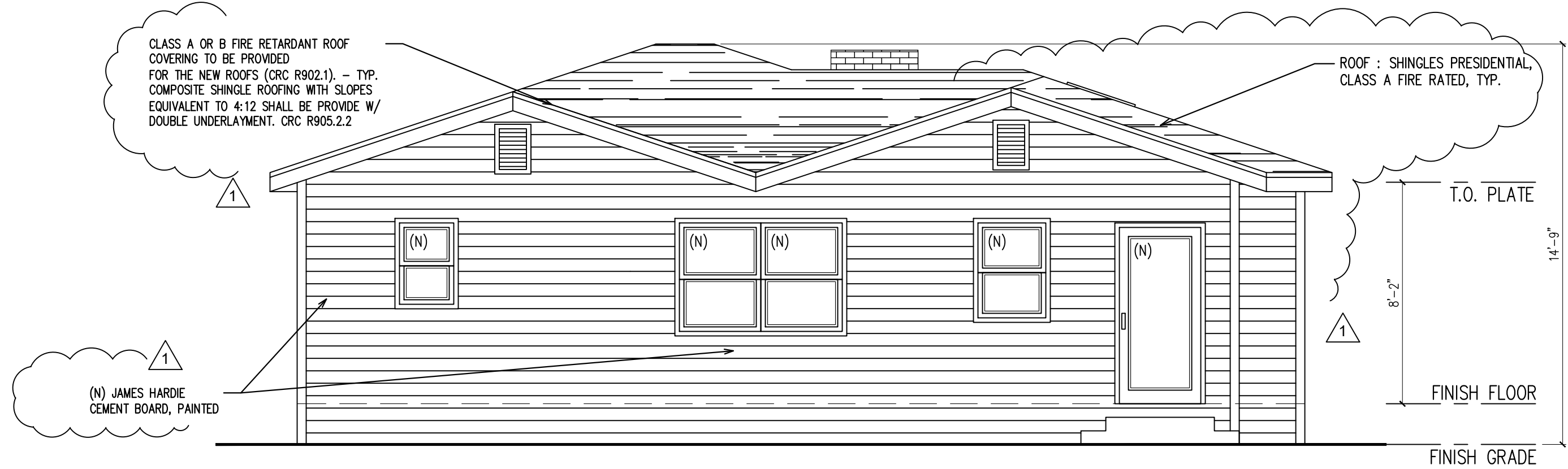
2 PROPOSED REAR ELEVATION SCALE: 1/4" = 1'-0"
