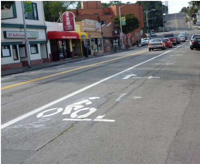
Figure 16. Use of parking T's along Class II and Class III bikeways to help bicyclists identify and steer clear of the “door zone” of parked vehicles. (source for diagram: City of Oakland)
