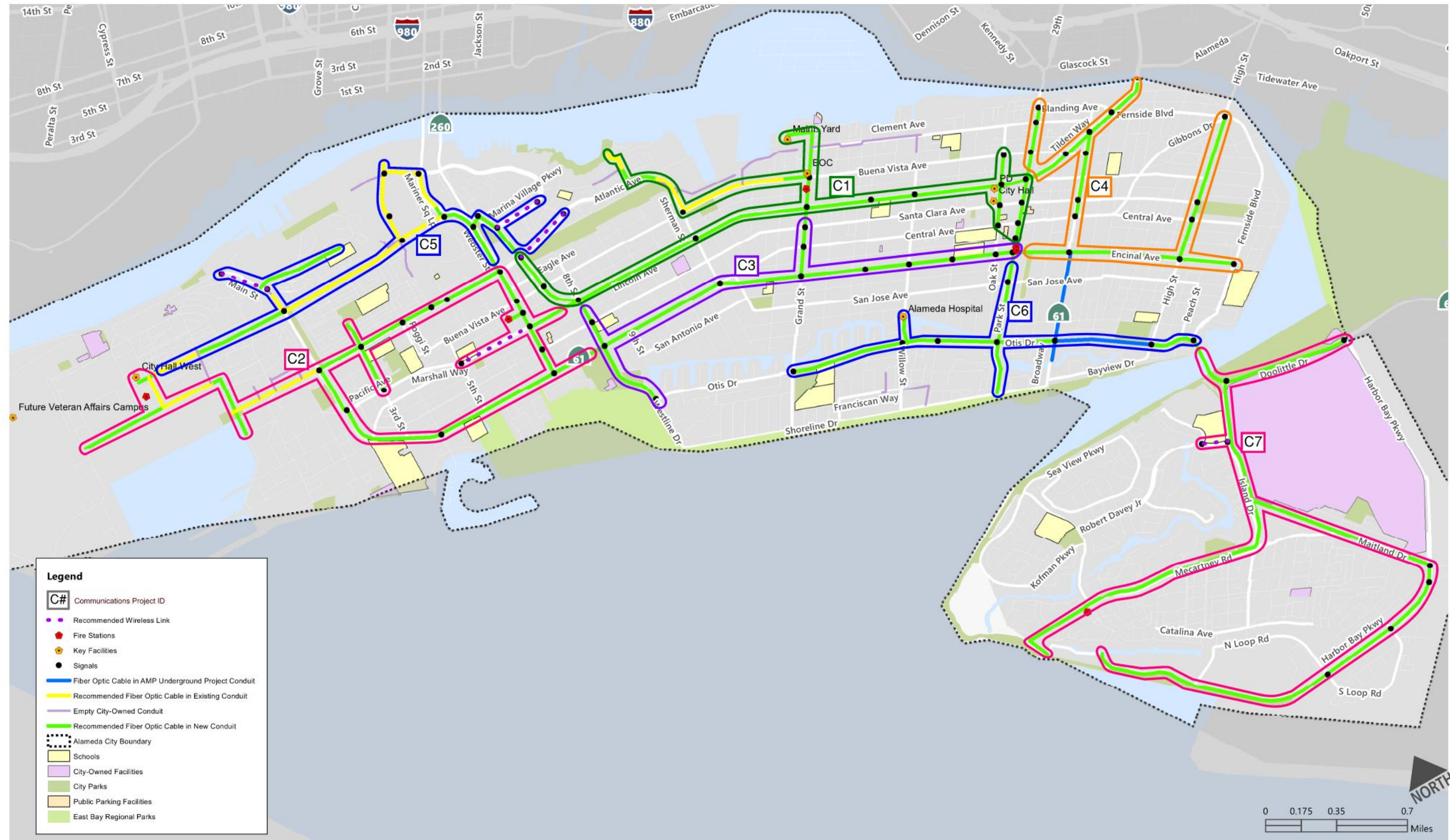
Figure 12: Proposed Communications Network Projects (Foundational Projects)
