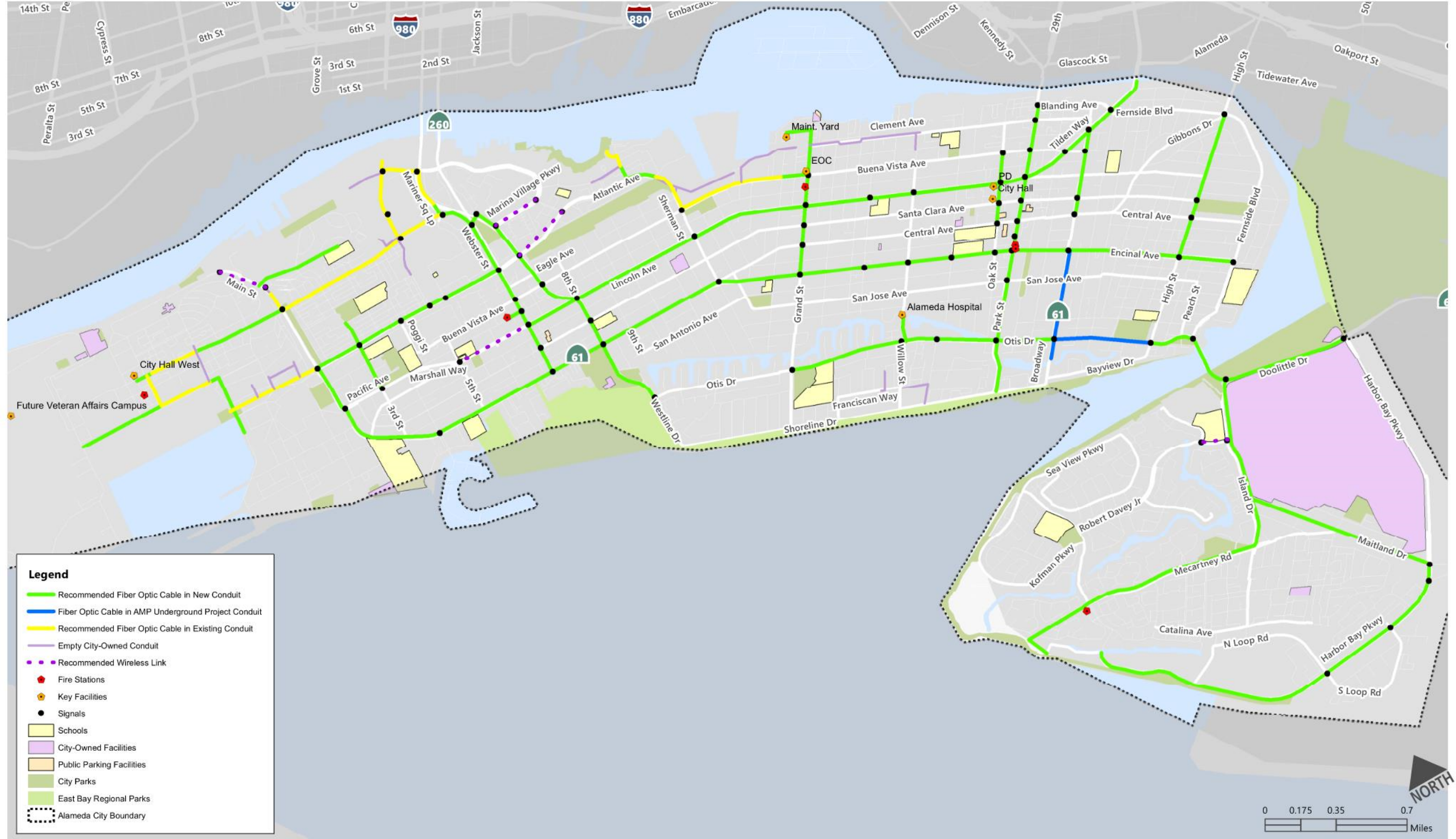
Figure 8: Recommended Communication Network Infrastructure
