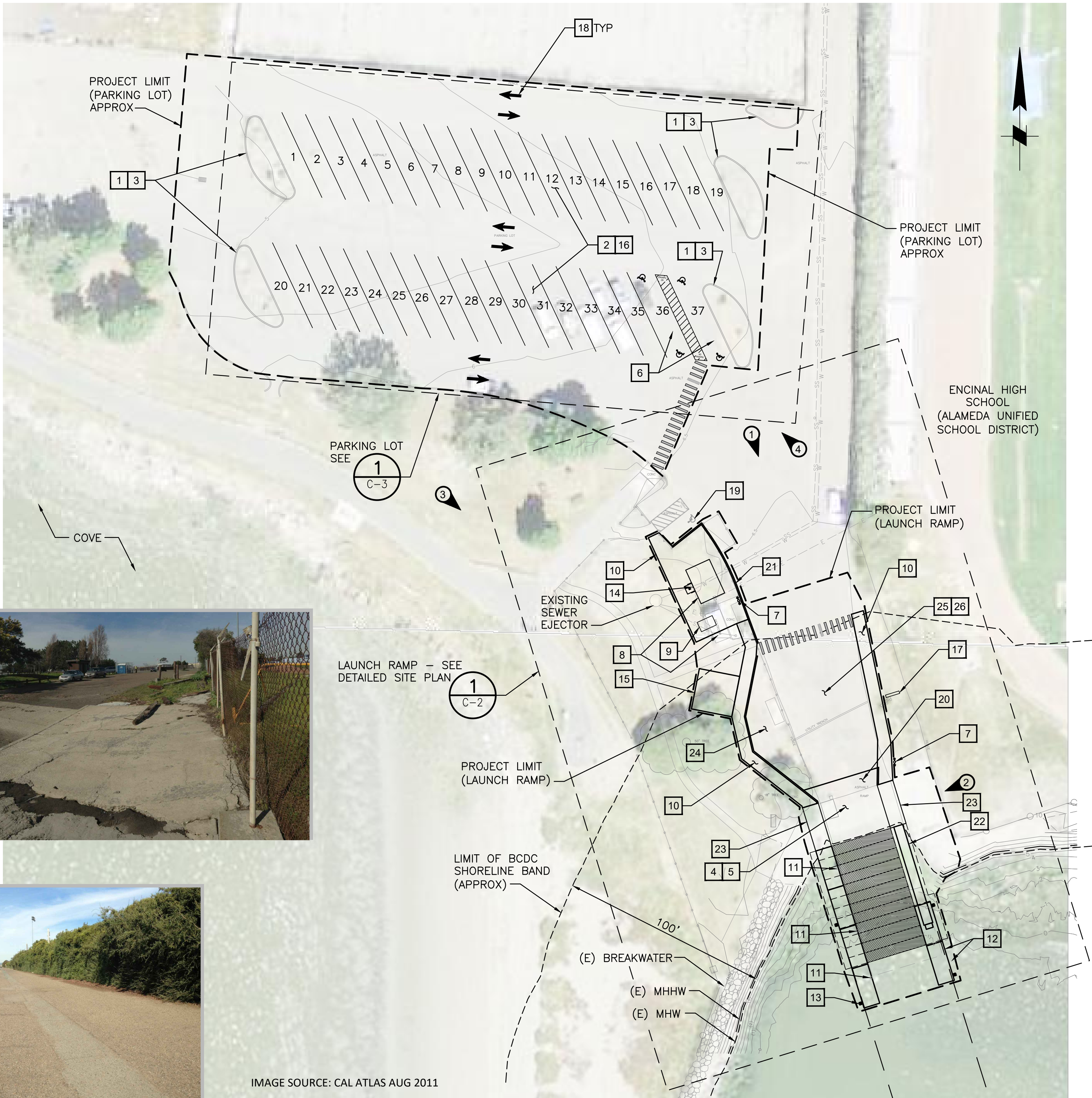
1 OVERALL SITE PLAN C-1 SCALE: 1" = 30'
