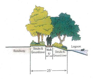
TYPICAL SECTION AT LAGOON EDGE Section F-1
