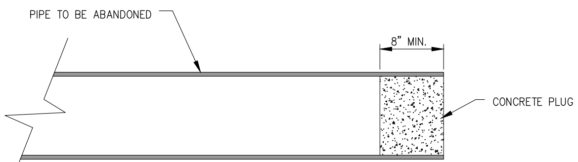
10" DIAMETER PIPE AND SMALLER
