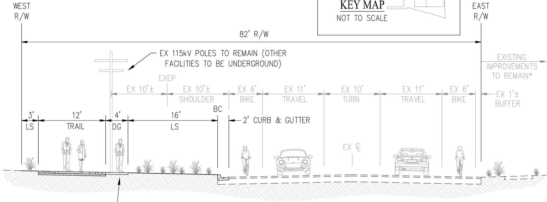
DG PATH TO BE ALIGNED TO PROVIDE MIN 4' UNOBSTRUCTED TRAVEL AT EXISTING POLES
