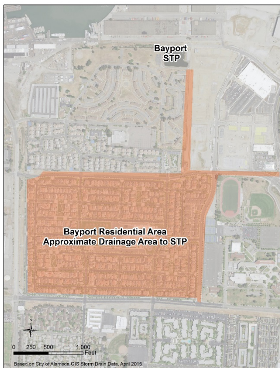
Figure 1. Approximate drainage area to Bayport STP from City Storm Drain GIS data dated April 2015
