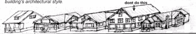
two story building out of scale with neighborhood.
